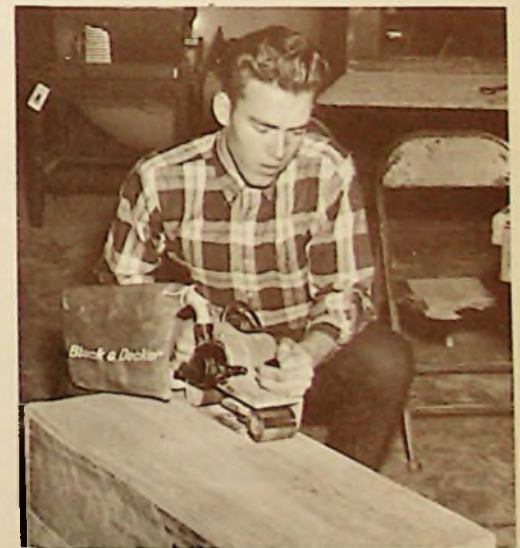
Utilizing the new portable belt sander, Sam Preston carefully smooths one side of his birch storage chest.
