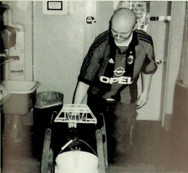
Casey Nolan gives his bridge a stress test during drafting class. The bridge was made from strips of balsa and held a total of 23 pounds before caving in. Maybe Casey will design the next bridge in Portsmouth.
