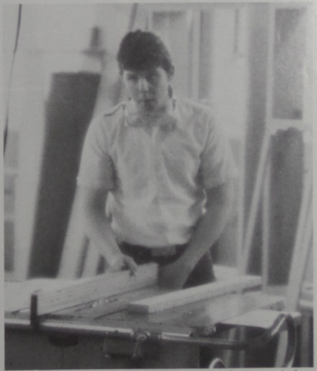
Heath Mefford adjusts the ripping fence on the circular saw before cutting a piece of pine in shop class.
